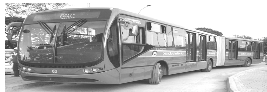
Figura 1. Bus articulado prototipo RENNO 280 GA Figure 1. Articulated bus prototype RENNO 280 GA
